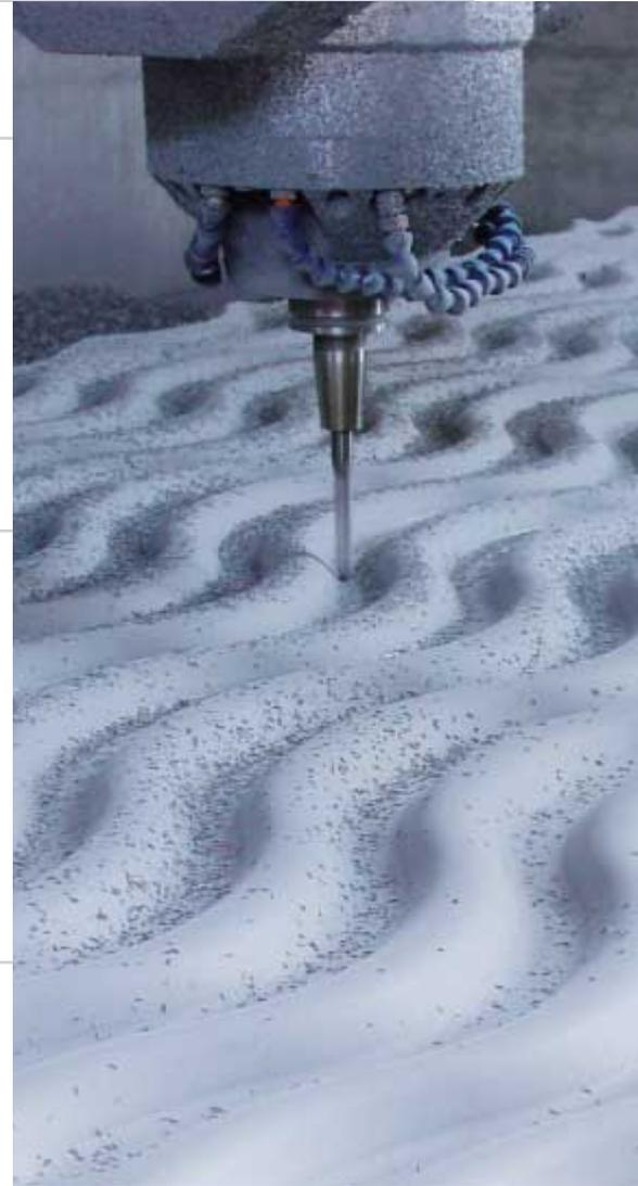
Vacuum forming mould of **ebablock**<sup>®</sup> W
