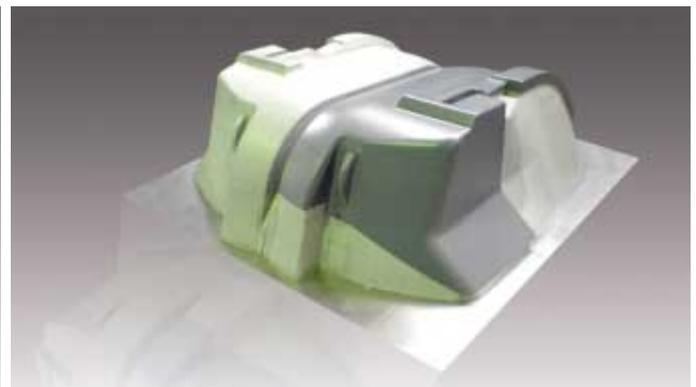
Vacuum forming double tool of **GH 705** (1200 x 1200 x 400 mm<sup>3</sup>)
